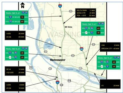
ODOT. In the Vancouver region, it provides real-time travel information to the public along the I-5, I-205, and SR-14 corridors. The project consists of white on green guide signs showing travel times to specific destinations via alternate routes and variable message signs with travel times to destinations along a route.
